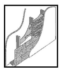
There are other beneficial considerations for using reflective insulation. Generally, these products have a very low water vapor and air permeance. When installed properly, with joints taped securely, reflective insulation materials are efficient vapor retarders and an effective barrier to air and radon gas.
