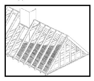
A Typical Attic Installation for Reflective Insulation
