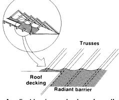
A radiant barrier can be draped over the ted to, roof sheathing trusses with the foil facing down.
