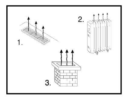
Typical examples of heat transfer through convection:
