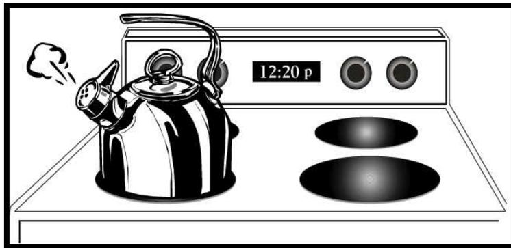
A typical example of conduction would be the heat transferred from hot coffee, through the cup, to the hand holding the cup. Another example, as shown above, the contents of the kettle boils from heat transferred from the burner to the kettle. Also, a poker becomes hot from contact with hot coals.
